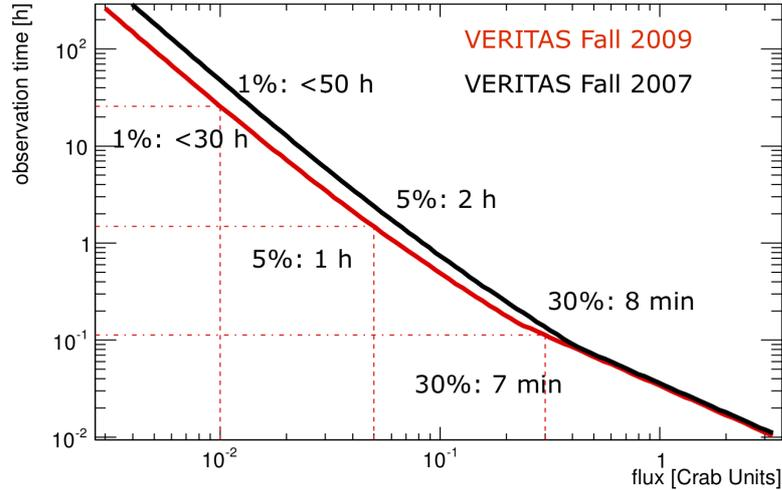
Fig. 2. VERITAS sensitivity before and after the move of telescope 1 and implementation of an improved mirror-alignment tool..
