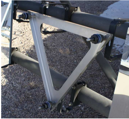
(a) Triangular three-point suspension mirror mount.
