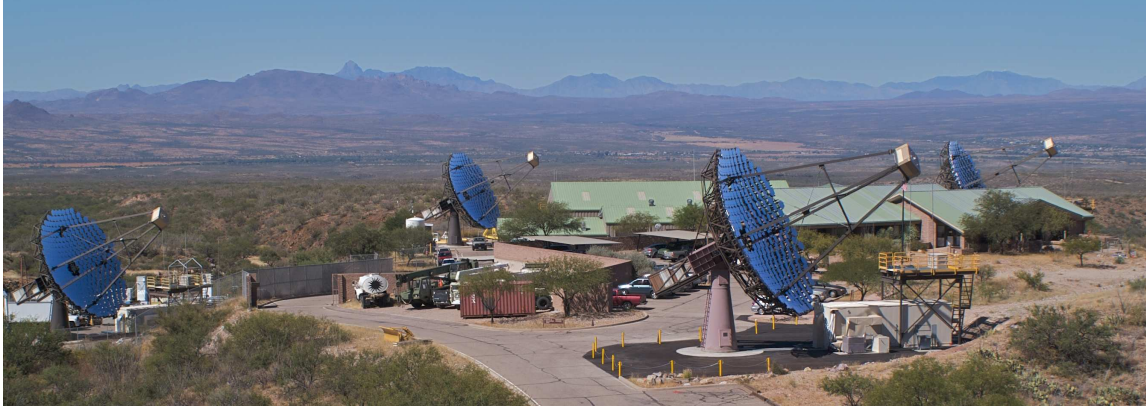
Figure 1–2: Image of the VERITAS Telescope Array in September 2009. The VERITAS array consists of four VHE gamma-ray telescopes and is located at the Fred Lawrence Whipple Observatory, in Amado, Arizona, USA.
