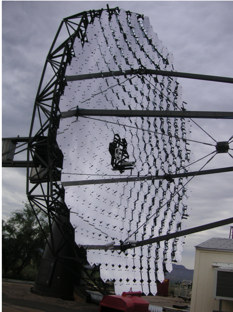
Figure 6.3: A picture of one of the VERITAS telescopes which shows the segmented mirror facets and the tubular steel OSS.
