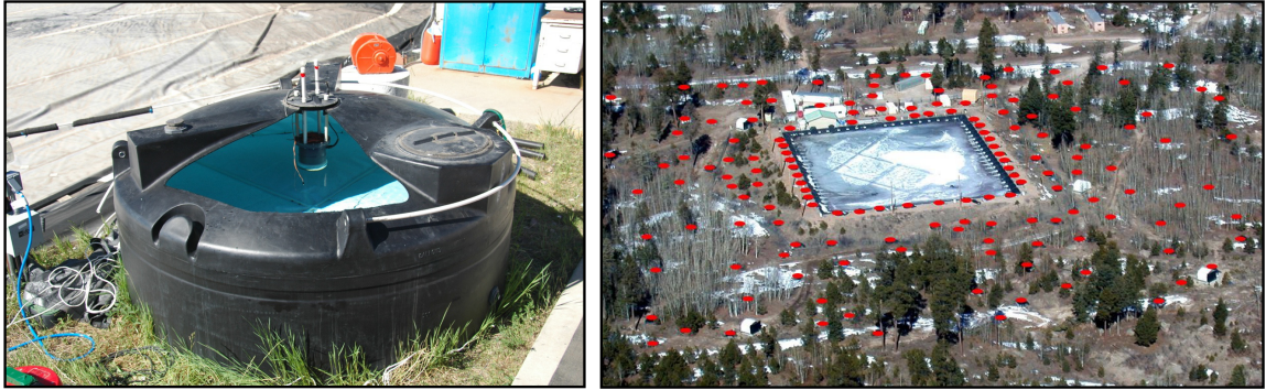
Figure 2.3: Left: A cut-away view of one of the Milagro outrigger tanks partially emptied of water but with the PMT still mounted inside. Right: An overhead view of the Milagro Observatory. The covered pond is in the center and the locations of the outrigger tanks marked in red.
