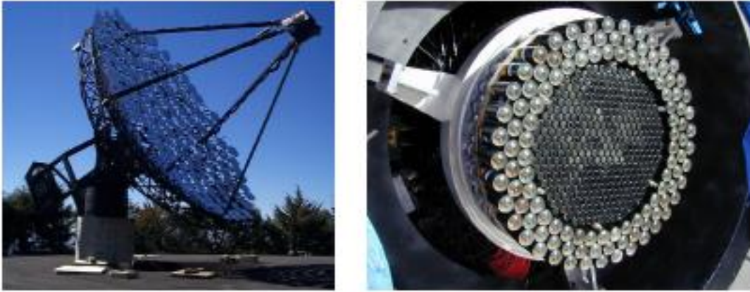
Figure 3.1 Whipple 10m and its focus-box. Left: Whipple 10m. Right: The 490 pixel camera in the focus-box, inner 379 PMTs are 0.5 inch in diameter, and outer 111 are 1 inch in diameter. The light-cones (absent when this picture was taken) are usually attached in front of the inner PMTs (figure taken from [11], Page 37).
