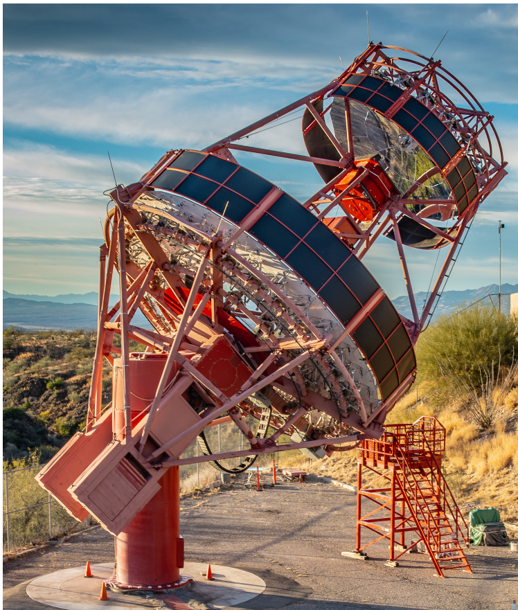
Figure 3.14: The prototype Schwarzschild-Couder telescope installed at the Fred Lawrence Whipple Observatory, from C. B. Adams et al. (2021).
