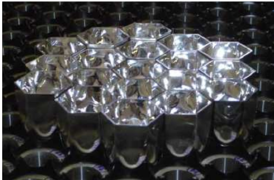
Figure 3.7: A view of the Winston light cones on top of the PMTs in the VERITAS camera. In normal operation, all PMTs are covered with light cones. From the VERITAS webpage, https://veritas.sao.arizona.edu/about-veritas/atmospheric-cherenkov-technique-and-veritas-technologies .
