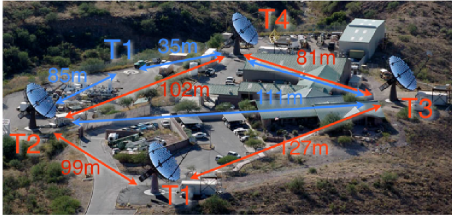
Figure 6: The locations and distances between telescopes both before the relocation of T1 (Blue) and after (Red)
