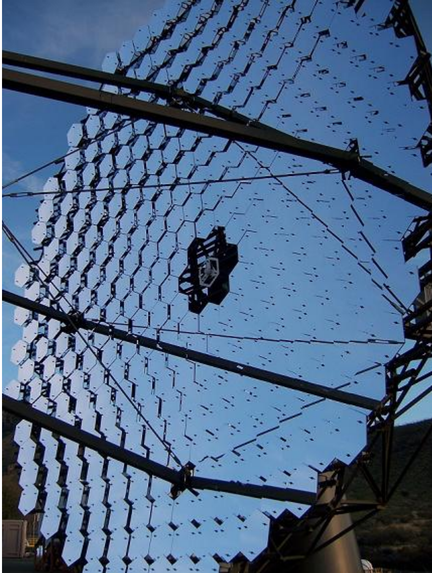
Figure 7: An image of a VERITAS telescope showing the mirror structure.
