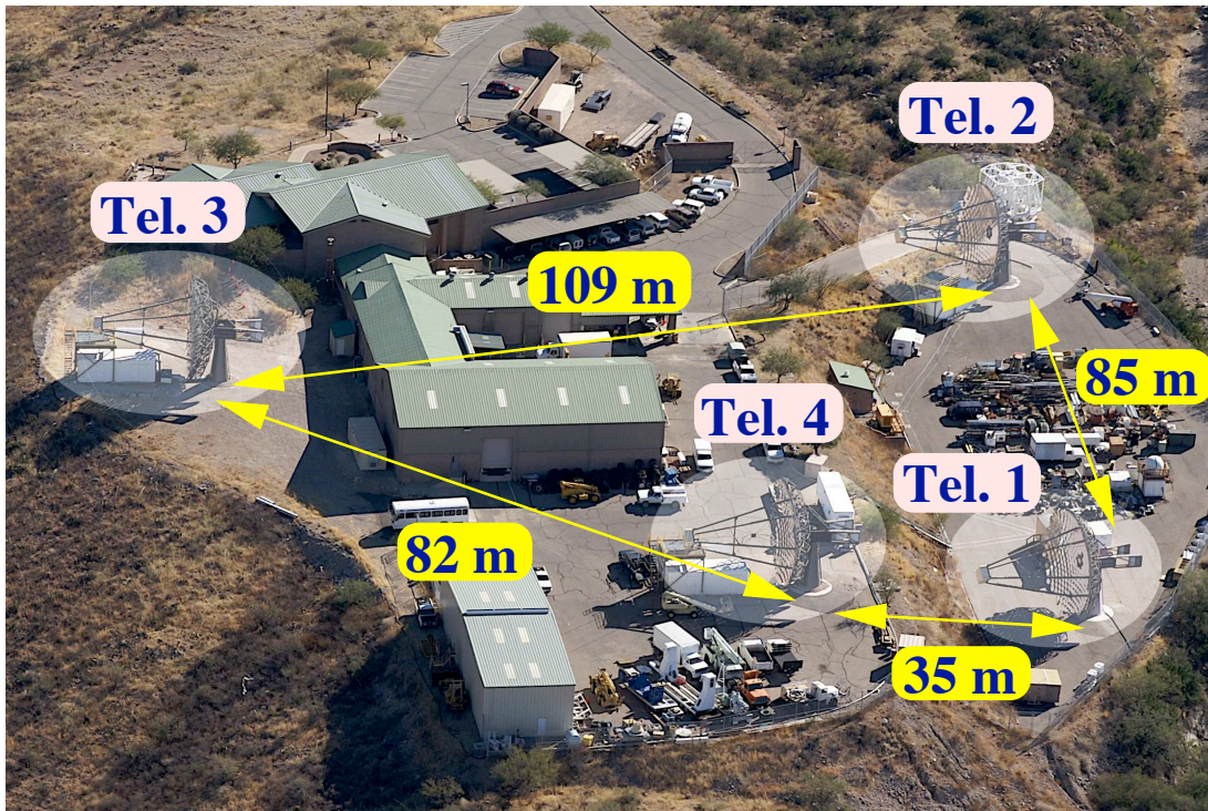
Figure 4.8: View of the VERITAS telescope layout at the FLWO basecamp showing the numbering of telescopes and their separations at the time when the dataset was recorded. More recently, in order to improve sensitivity, the telescope labeled as ‘Tel. 1’ has been moved.
