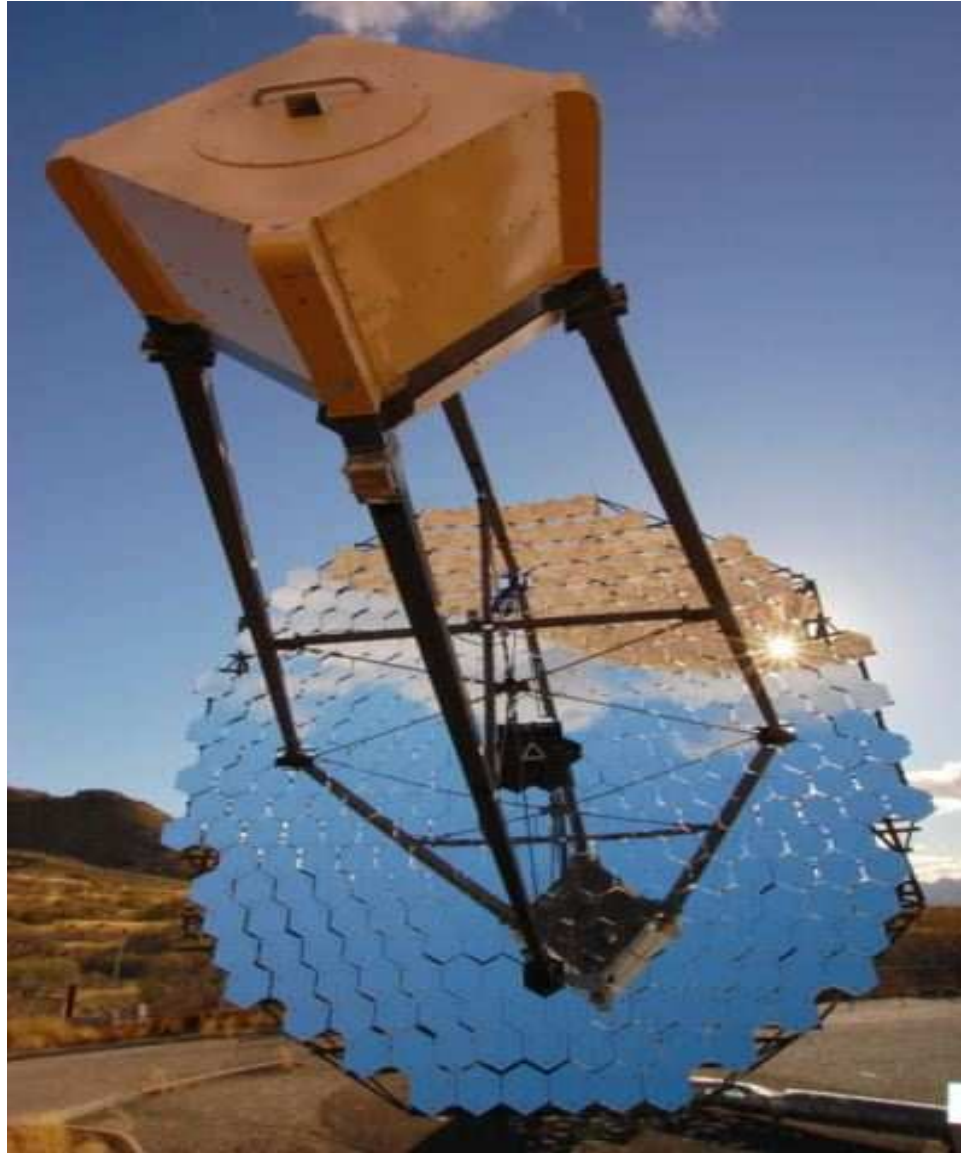
Figure 3.4: A front view of the T2 reflector. The reflector is made by close packing the 345 small hexagonal mirrors.
