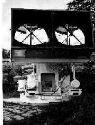
Fig 2.11: The second ground-based gamma-ray telescope, the British-Irish experiment at Glencullen, Ireland (1964). The telescope consisted of two 90 cm searchlight mirrors on a Bofors gun mounting. The experiment was led by Jelley and Porter.
