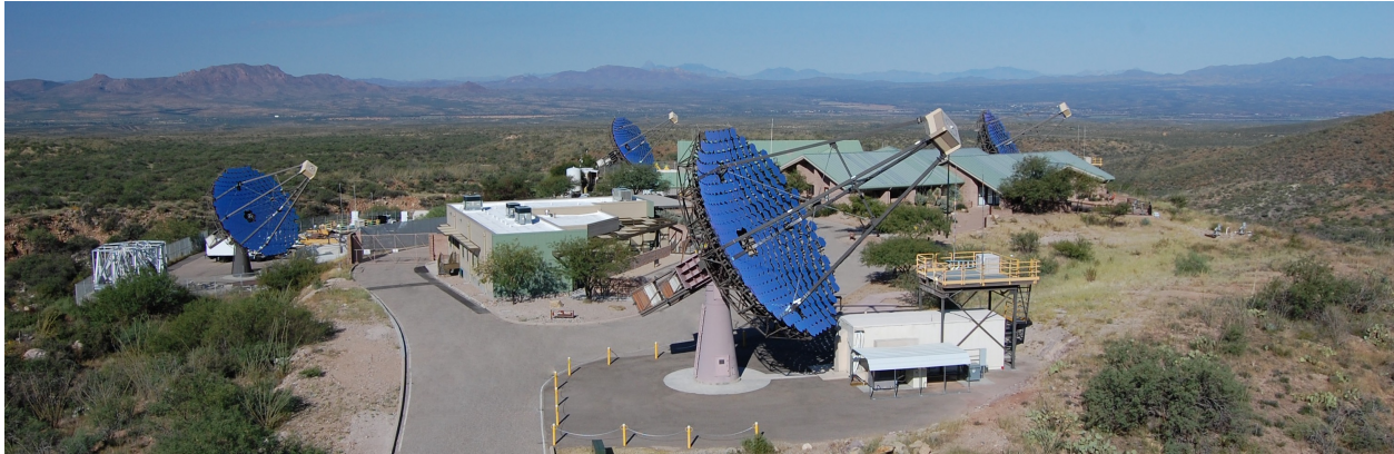
Figure 3.1. Photograph of VERITAS’s four 12 meter diameter imaging atmospheric Cherenkov telescopes. VERITAS is located at the Fred Lawrence Whipple Observatory at the base of Mount Hopkins in southern Arizona. Image credit: Larry Ciupik.
