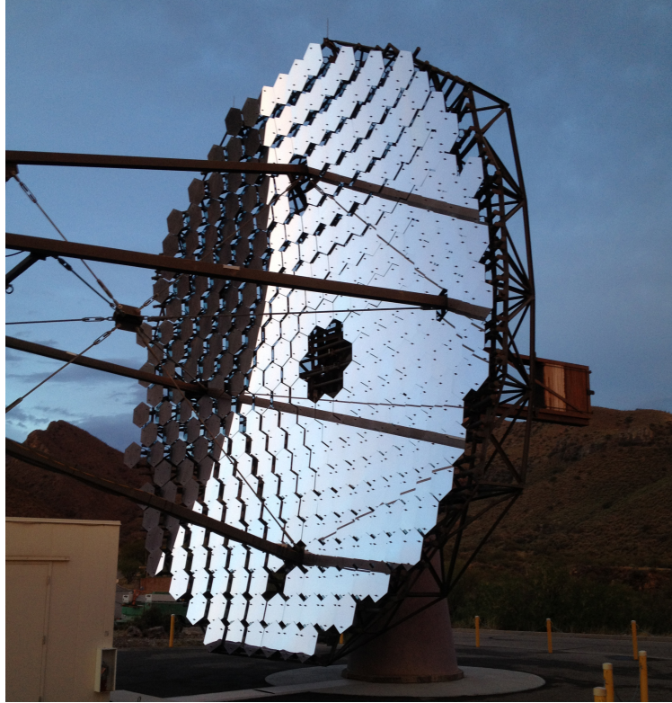
Figure 3.5. Photo of VERITAS telescope 1 showing the Davies-Cotton reflector.
