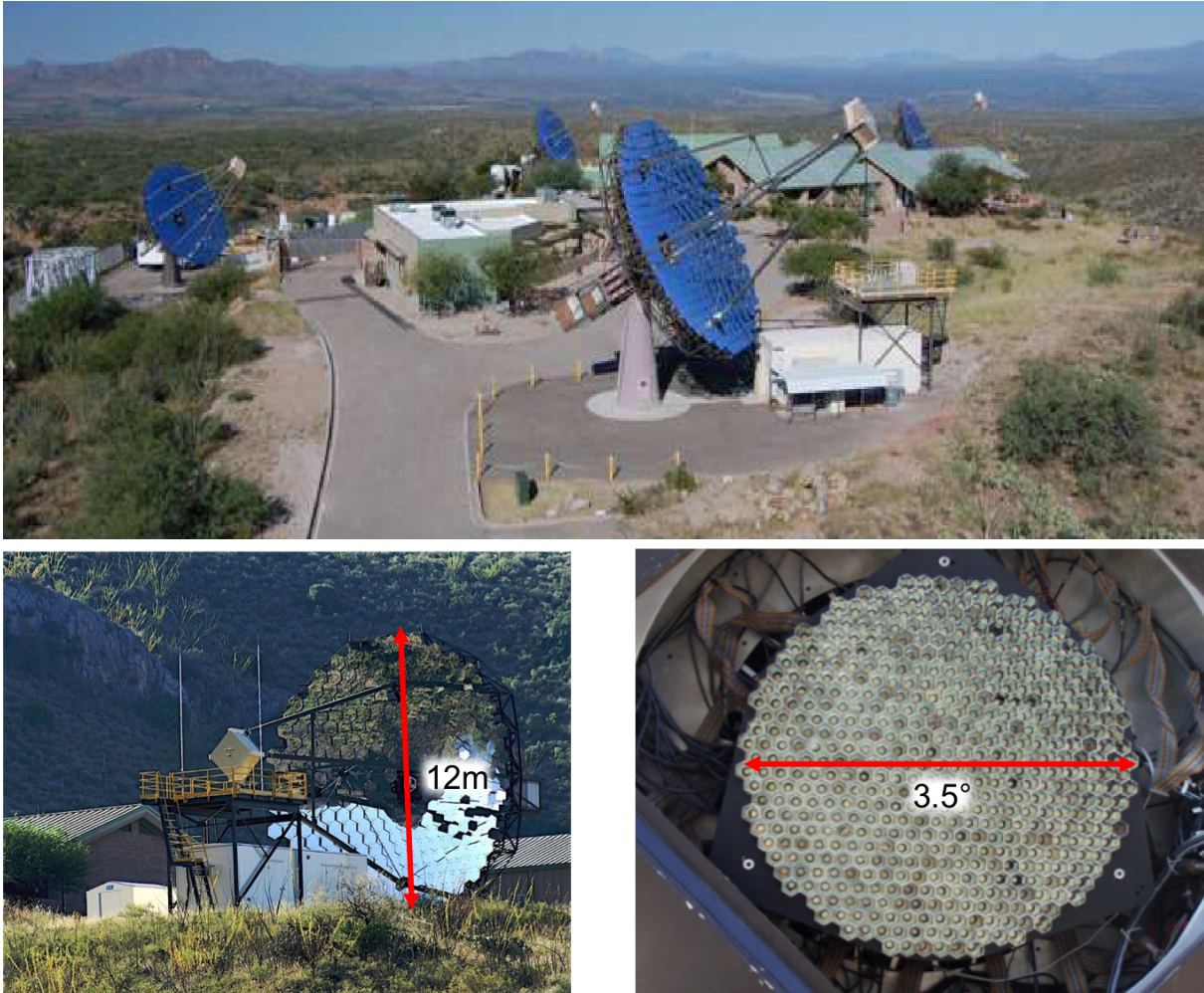
FIGURE 1.6: Top: A panoramic view of Whipple Observatory Base Camp in Southern Arizona, containing the VERITAS array. From Sentürk (2013) . Bottom: An image of a single telescope of the array as well as its camera. The diameter of the telescope is 12 meters. The camera consists of 499 photomultiplier tubes corresponding to a field of view of approximately 3.5^\circ . From Holder (2015) .
