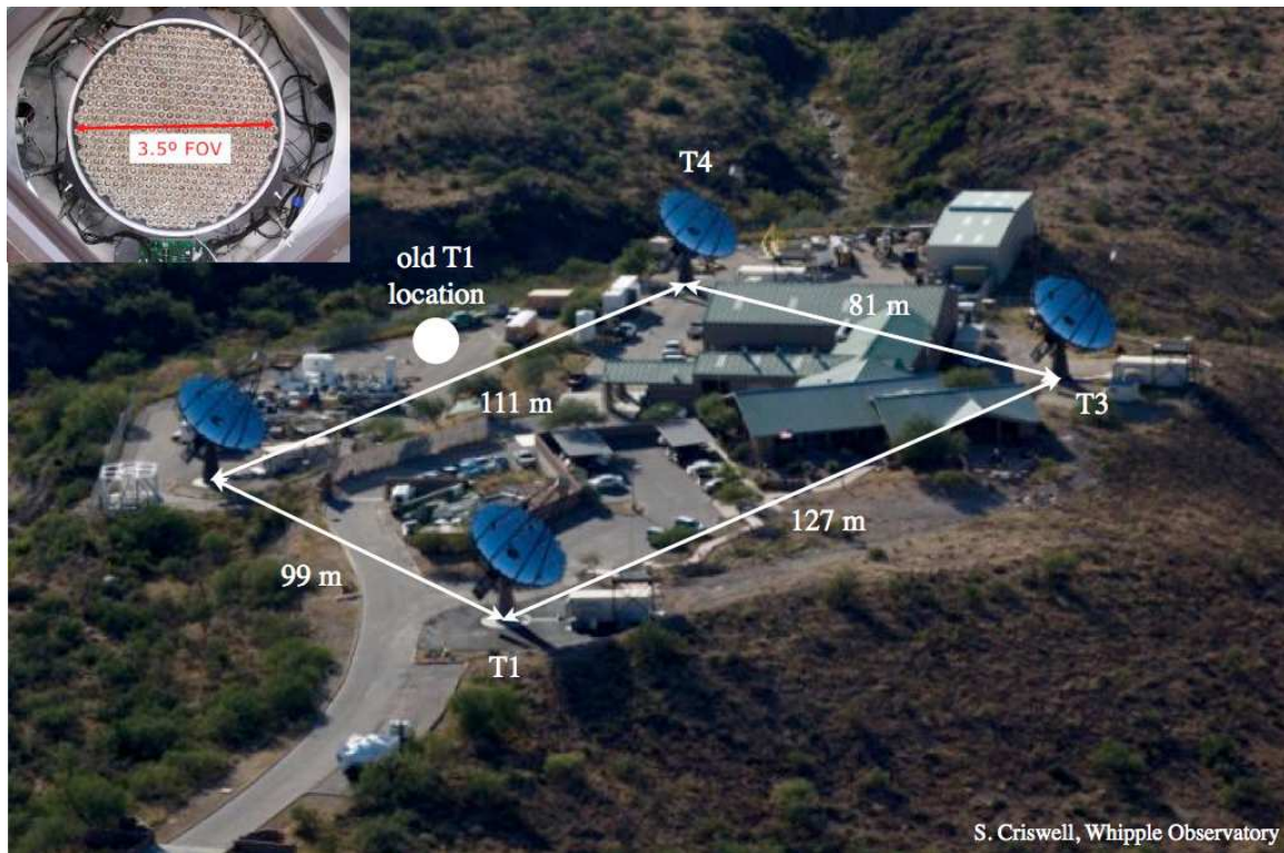
Figure 3.5. Aerial view of the VERITAS array on Mount Hopkins, Arizona. Top left insert shows a closeup picture of the 3.5^\circ FOV camera on each telescope.
