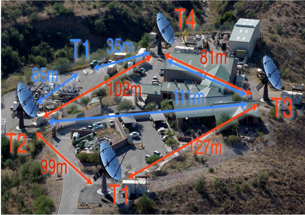
Figure 3.1: An illustration of the old telescope layout (blue) and the new telescope layout (red). The difference being that Telescope 1 was moved 200 m eastward from its initial position.
