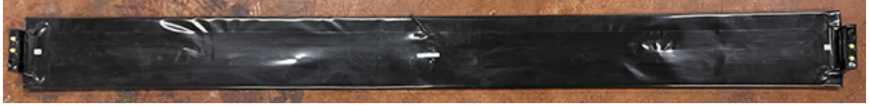
Figure 17: Photograph of a single constructed 1.8 m paddle. Relative sizes of the scintillator and preamp enclosure can be seen. Black plastic covers the entire assembly. We define the long (horizontal) axis as the x axis.
