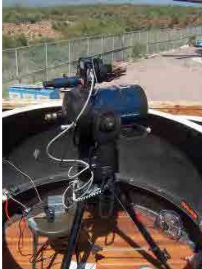
Figure 4: Atmospheric Monitoring System
