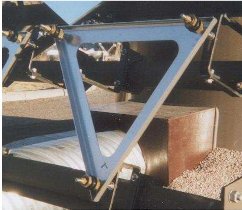
Figure 5.5: A picture of an individual mirror facet mount clearly showing the mounting bolts for the mirror facets.
