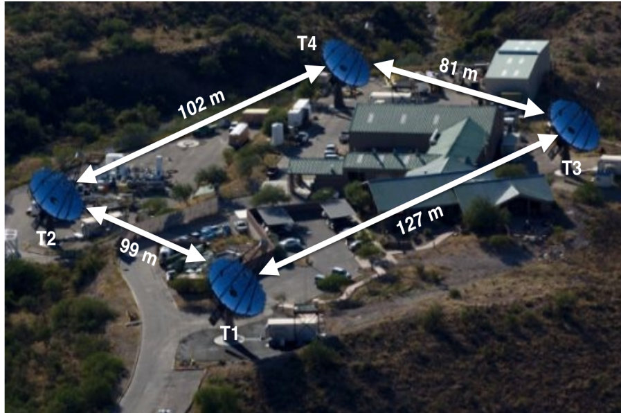
Figure 3.1: Array Layout of VERITAS Observatory
