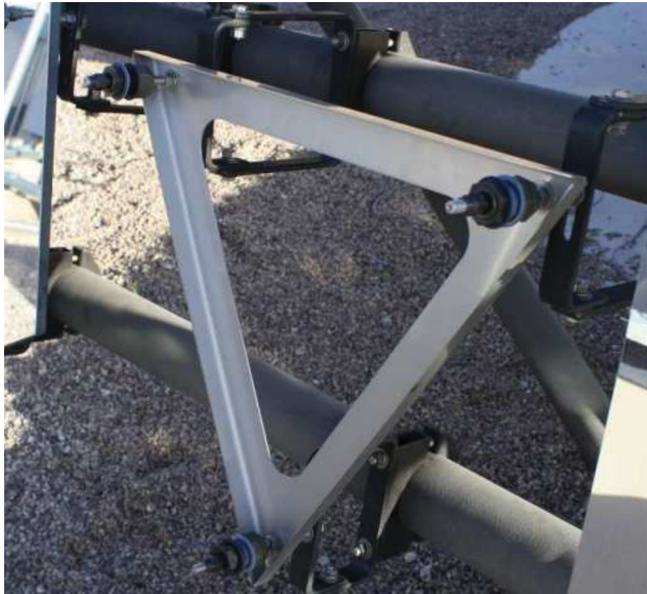
Figure 3-3: Picture of a VERITAS mirror mount. Each of the three points of the mount consists of a mounting bolt, a fine-alignment screw and a gimbal. Image credit: Andrew McCann.
