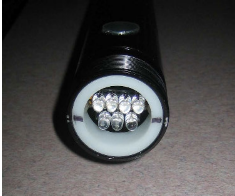
Figure 3.29 An example of the LED flashers currently used to take VERITAS calibration runs.
