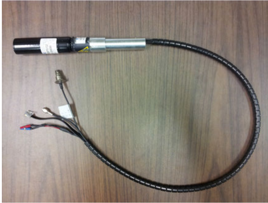
Figure 3.19 A Photonis XP 2970/02 pixel. These pixels comprised the VERITAS photodetector system from the beginning of operations until the summer of 2012.
