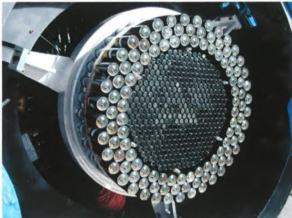
Figure 3.3: The Whipple camera with 490 photomultiplier tubes.
