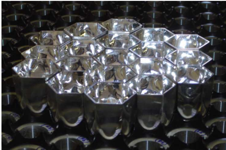
Figure 3.10: A sample of the hybrid Winston cones used to construct the light-concentrator faceplates. Image credit — Fig. 7 of [168].
