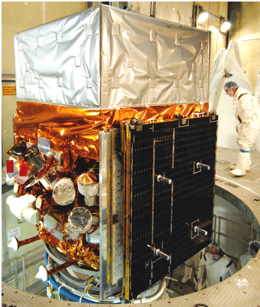
Figure 1.5: The Gamma-ray Large Area Space Telescope before launch, after which it was re-named the Fermi Gamma-ray Space Telescope, in honour of Enrico Fermi. On the right are folded solar panels; on top is the Large Area Telescope covered by thermal blankets which also provide protection against micrometeors. Image credit — Fermi /NASA.
