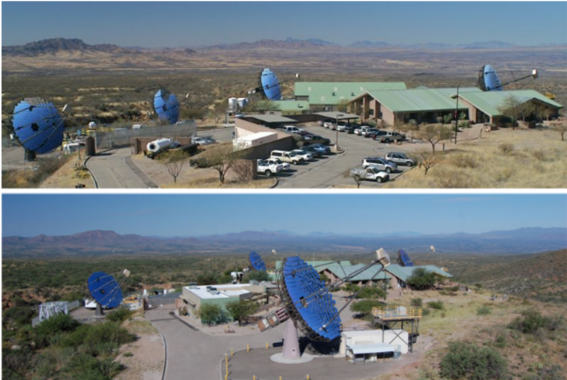
Figure 2.4: The top panel shows the V4 configuration of VERITAS, prior to the relocation of T1. The V5 configuration is shown in the bottom panel for comparison, where the array forms a more uniform quadrilateral. This configuration provides improved background rejection capabilities, increasing the overall sensitivity of VERITAS by \sim 30\% . The time required to detect a source of 1% Crab Nebula flux at the 5\sigma level decreased from 48 hours to 30 hours.
