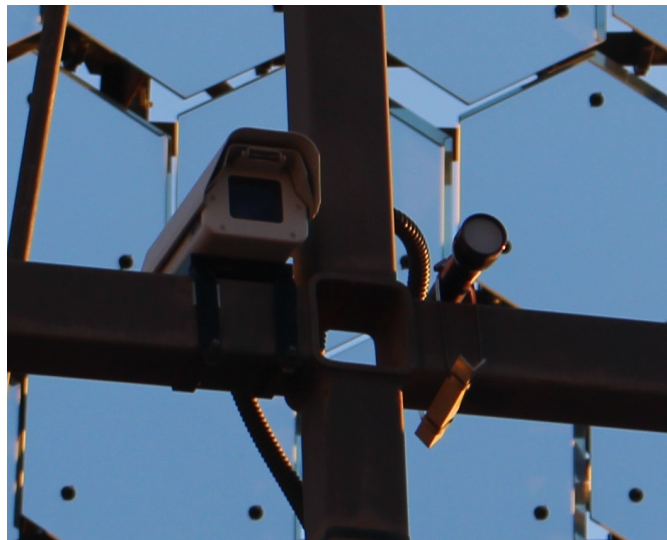
Figure 3.6.: The VPM (white box) that monitors the positions of the LEDs in the camera box to allow for correction due to deflection in the OSS. Besides the VPM camera is the flasher assembly contained inside a modified torch.
