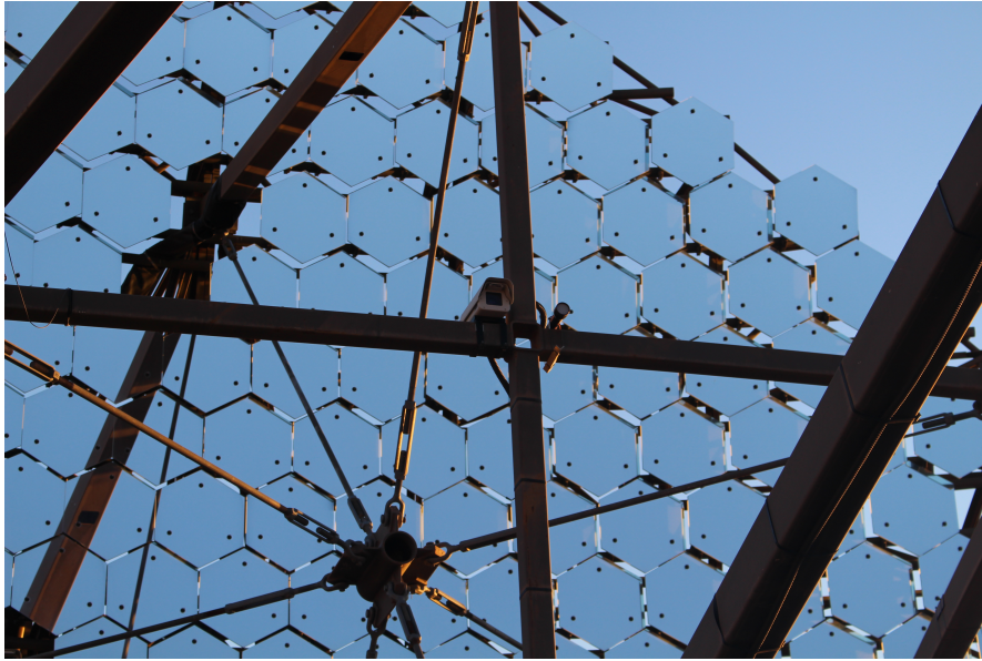
Figure 3.2.: A section of the hexagonal mirrors on a VERITAS telescope. Each mirror is mounted on three custom mounts to allow for accurate alignment. Also visible is part of the OSS that holds the camera.
