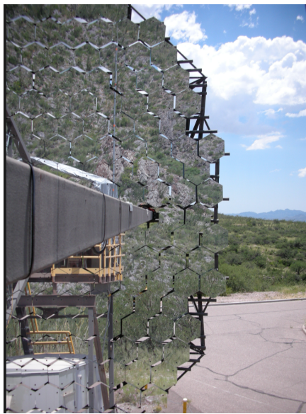
Figure 3.2. Hexagonal Mirrors of the VERITAS Reflector
