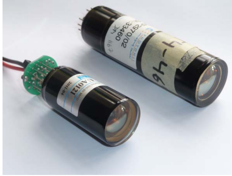
Figure 5.3: The pre- and post-upgrade photomultiplier tubes used in the VERITAS cameras. The Hamamatsu R10560-100-20 is shown in the bottom-left and the Photonis XP2970/02 in the top-right.
