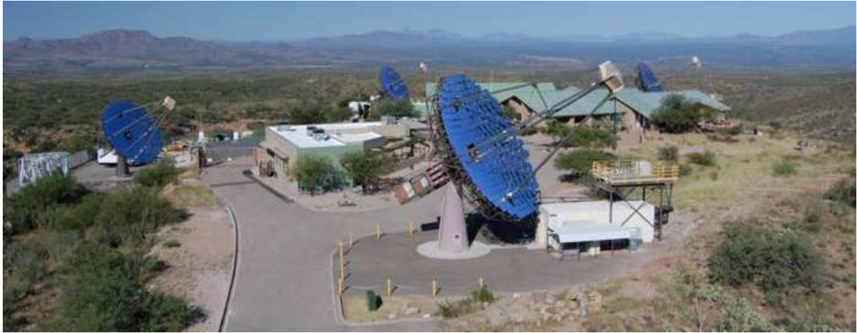
Figure 2.1: The VERITAS observing site. The array, composed of four imaging atmospheric Cherenkov telescopes surrounds the control building.
