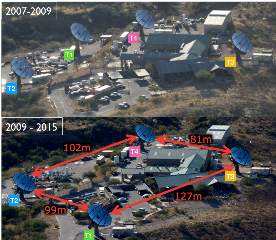
Figure 2.2: The layout of VERITAS array before ( top ) and after ( bottom ) the T1 move.
