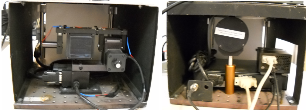
Figure B.1 The VERITAS alignment tool front (left) and rear (right) view.
