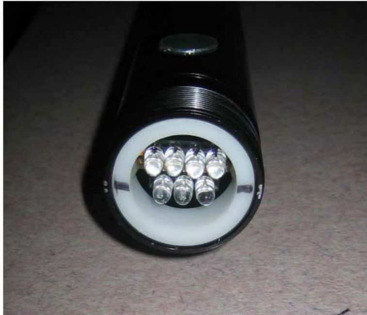
Figure 2-10: View inside the flasher with the diffuser removed (credit: Dave Hanna [126])
