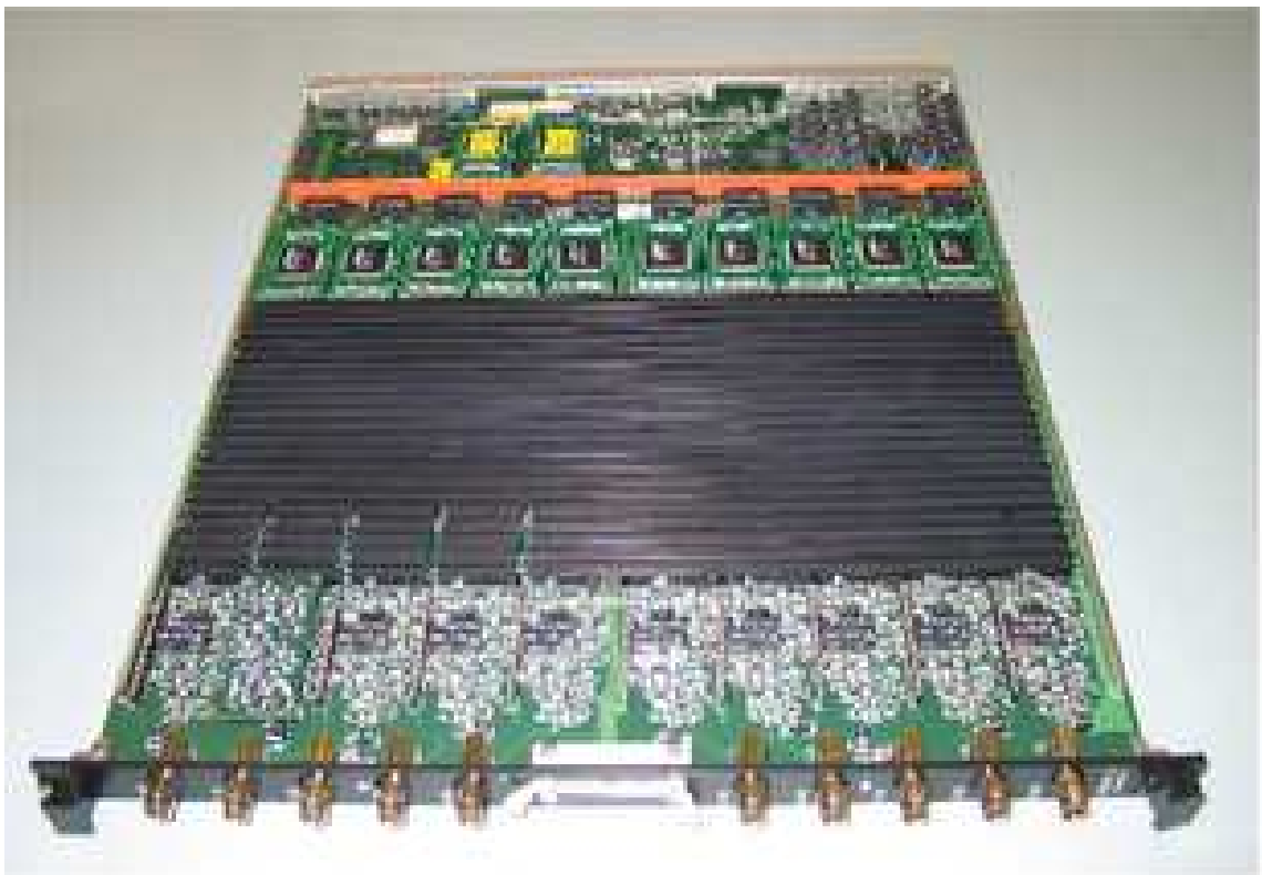
Figure 5.10: Photograph of a FADC board. One can see the 10 input channels receiving pulses from 10 pixels. Sitting on the board are also the CFD modules, one for each channel.
