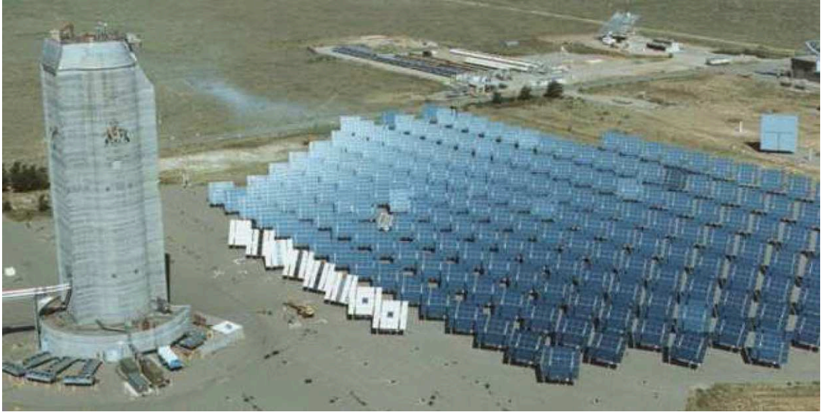
Figure 4.14: The STACEE experiment. A large field of heliostats reflects the Čerenkov light to an array of photomultiplier tubes placed on an observing tower. Figure taken from [1].
