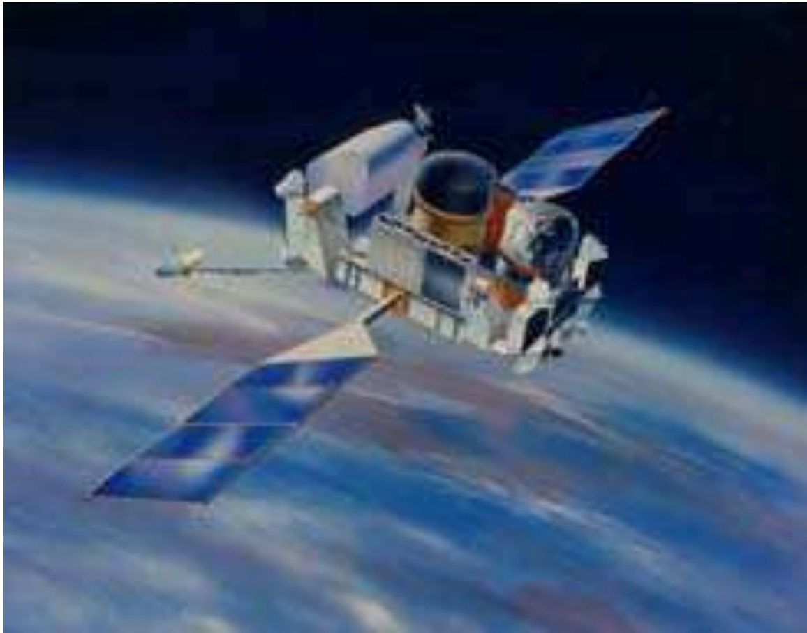
Figure 4.4: The CGRO satellite. It hosts four instruments: COMPTEL, BATSE, EGRET and OSSE. Figure taken from http://cossc.gsfc.nasa.gov/docs/cgro/ .
