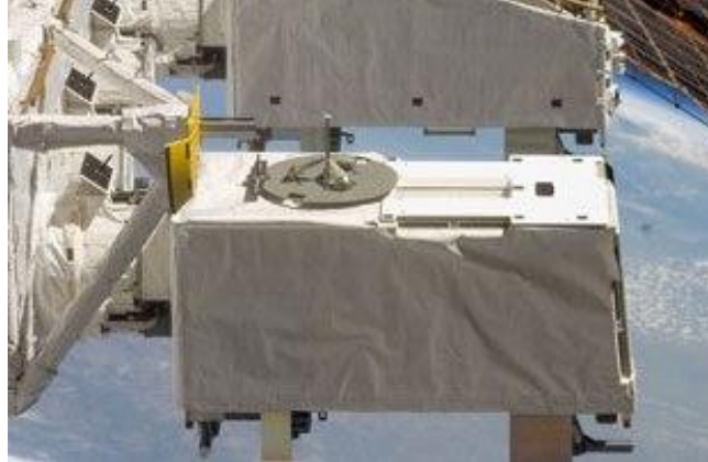
Figure 3.9.: View of MAXI on the Japanese Experiment Module - Exposed Facility (JEM-EF) on the ISS. Image credit: MAXI.
