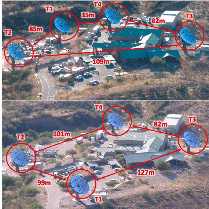
Figure 2.1 Image of the four telescope VERITAS array in its former (2007 - 2009; top ) and current geometrical layout (2009 - present; bottom ). Overlaid on the image is the identifying number of each telescope (T1, T2, T3, and T4) and the physical distances along the array perimeter. Photos courtesy of Steve Criswell, FLWO.
